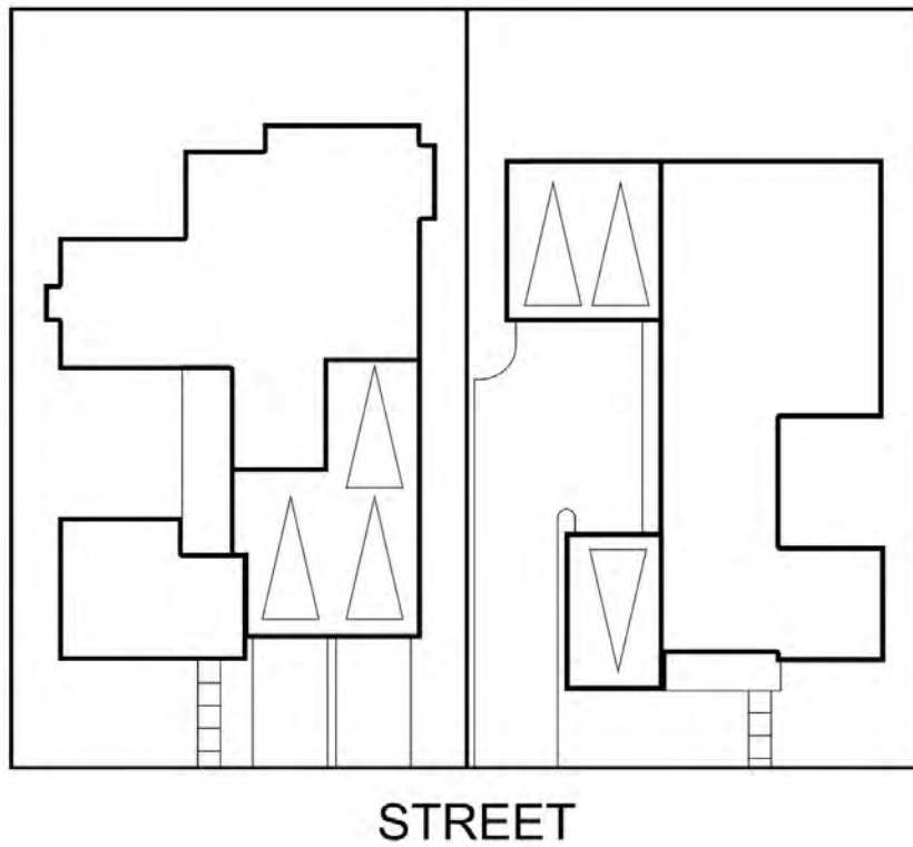
CONCEPTUAL BUILDING TYPE A & LOT SIZE: Single-Family Detached Front Loaded (60'x100') (subject to future City approvals)
